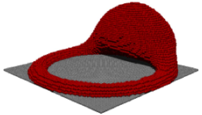
FIG. 14. (Color online) Bulge morphology obtained in N - V - T Monte Carlo simulations for a 30-40-ring-patterned surface. T/T_c = 0.86 , \alpha = 0.3 .
